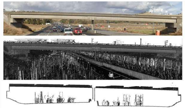
Extracting the surface, overhead power lines and poles from aerial surveys;
